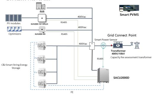
Huawei C&I Smart String Energy Storage (ESSs for short) Products LUNA2000B series are applicable to industrial and commercial scenarios. They work with the SmartPCS, DCDC and SACU. The SmartPCS is connected to the pack controller DCDC, and charges batteries when the power grid is sufficient. When the power grid needs to be output, the SmartPCS outputs the stored battery energy to loads for use.
